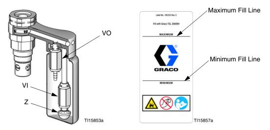
FIG. 11. Cutaway of TSL Reservoir, and Fill Lines
